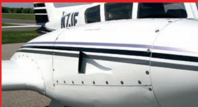
NACA Induction System (PA-30/39 Only) 2 mph
