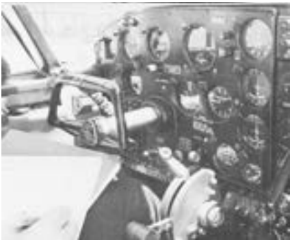
Modified power quadrant and addition of a “new breed” of engine gauges on panel alter the cockpit only slightly.
