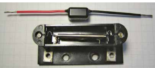
Figure 5: Open flasher housing with the solid-state flasher circuit.
