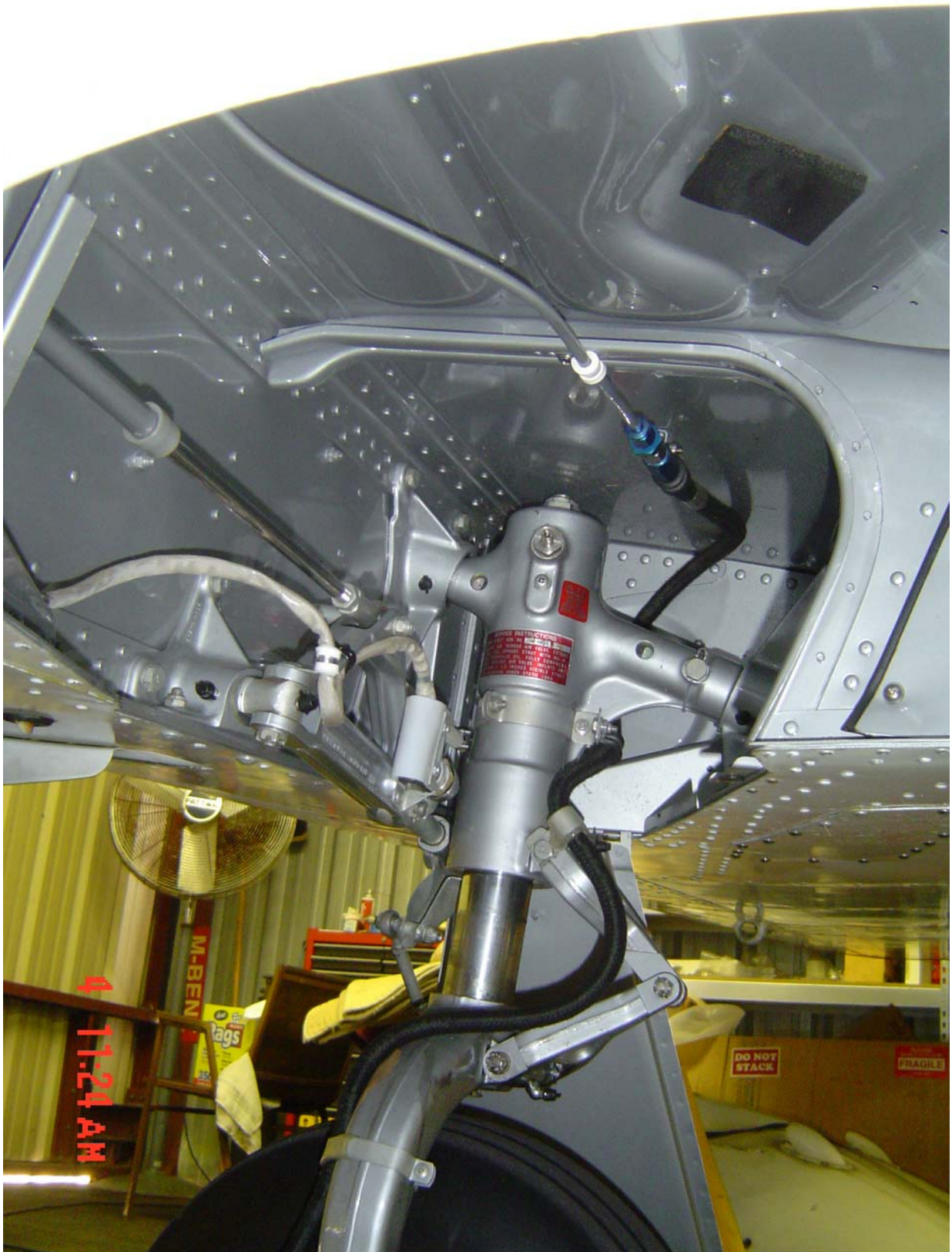
BRAKE HOSE CLAMPS LOCATIONS, RH
