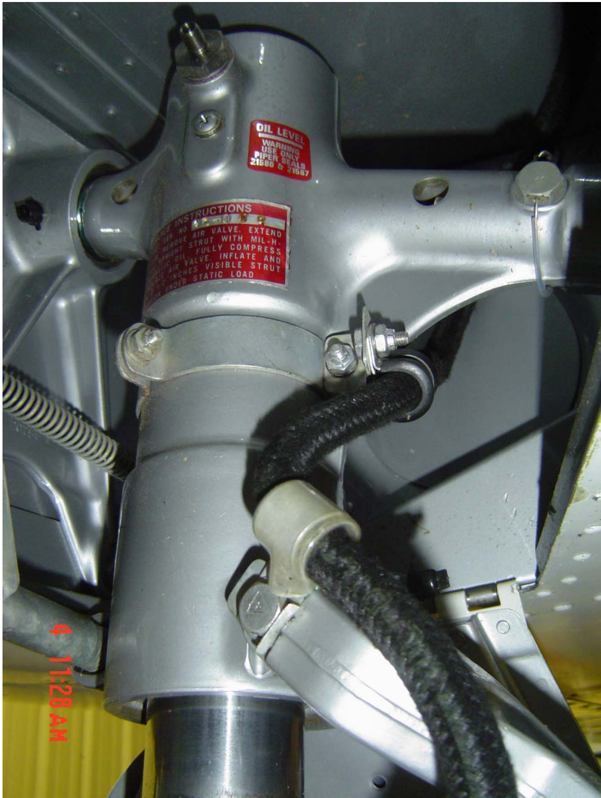
BRAKE HOSE CLAMPS LOCATIONS, RH
