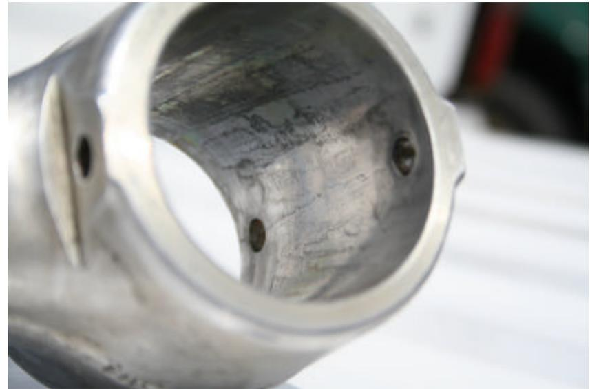
**NOTES: Cracks observed on singles only. Cracks only observed on early model singles (1958 – 1961). Forward cracks observed at ~3800 hours, while forward and aft cracks observed at ~4900 hours. Later models with higher times have not cracked. No cracks found on Twins or 400 Model singles.**
