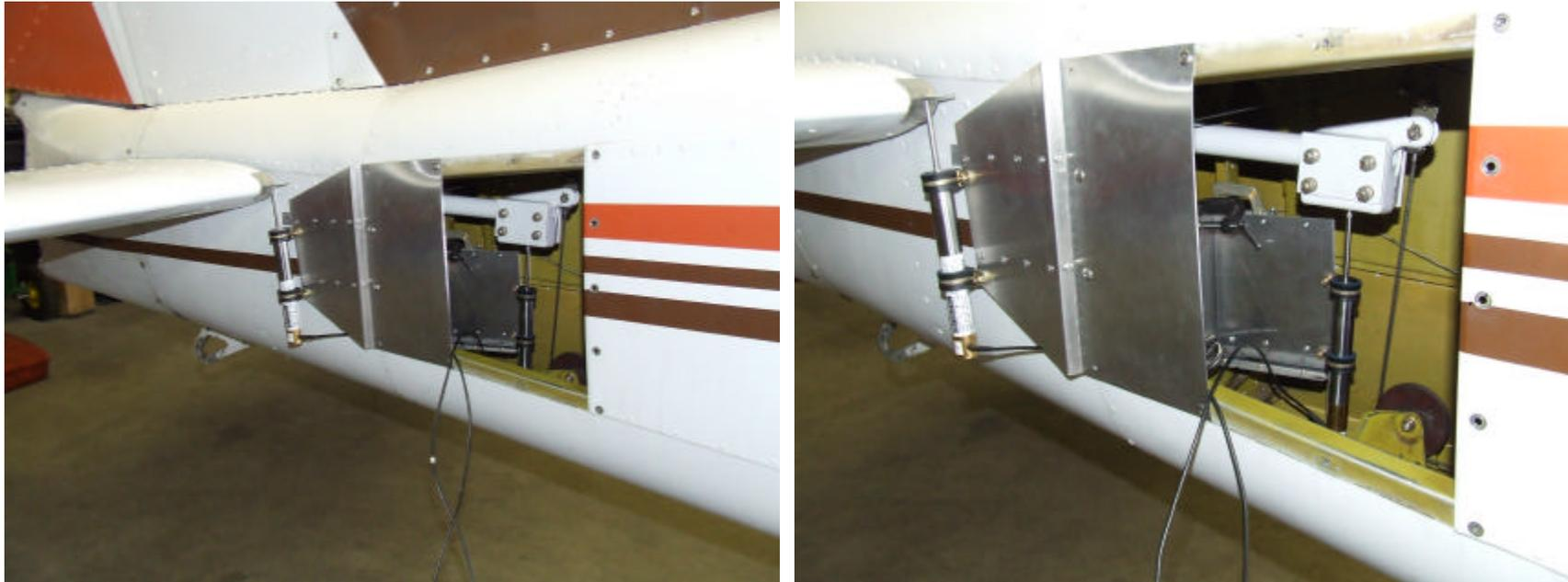
**Notes:** Brackets fabricated from aluminum sheet to support 5 KHz AC LVDT's measuring stabilator leading edge and counterbalance weight motion. Output to oscilloscope not successful. Data taken from digital displays (~.5 Hz refresh rate).
