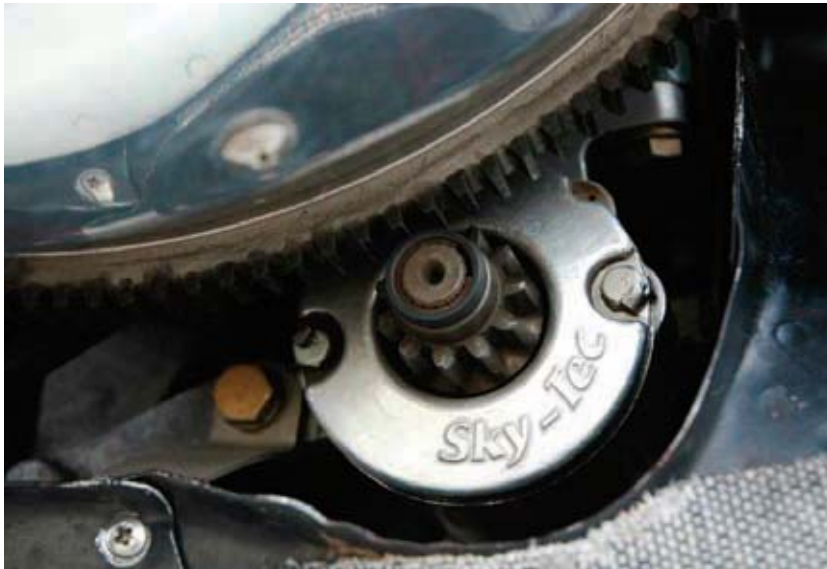
Front view of the Sky-Tec NL lightweight high torque starter
